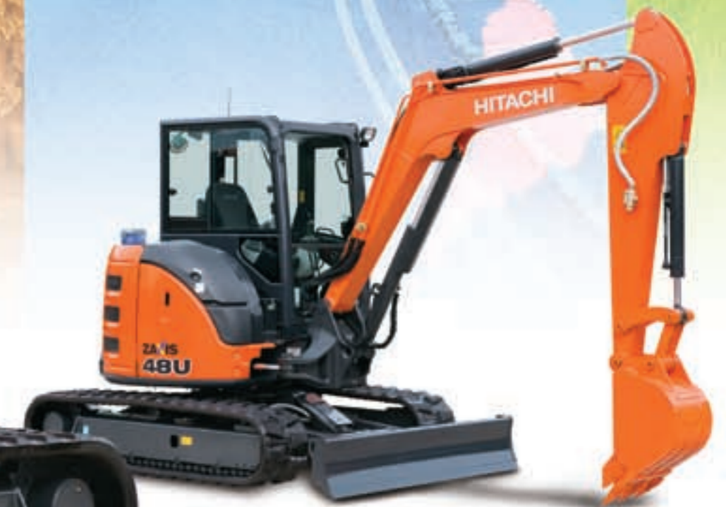
Shown equipped with 1.38 m arm, extra piping, additional counterweight, rear view mirror, and pre-cleaner.
