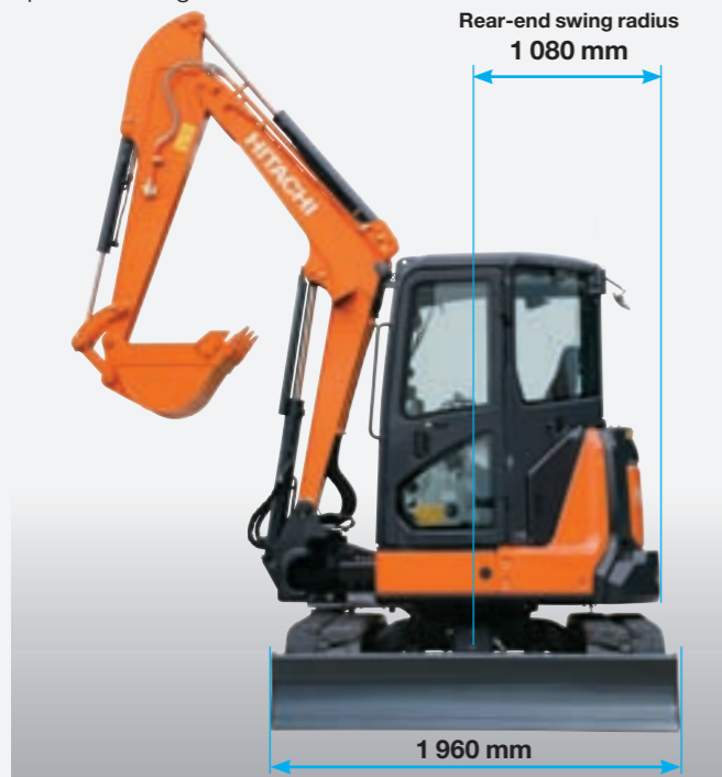
Shown equipped with 1.69 m arm, extra piping and additional counterweight.
